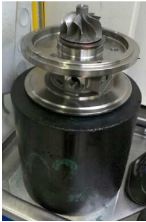
Fig. 1. Impeller mounted for magnetisation
