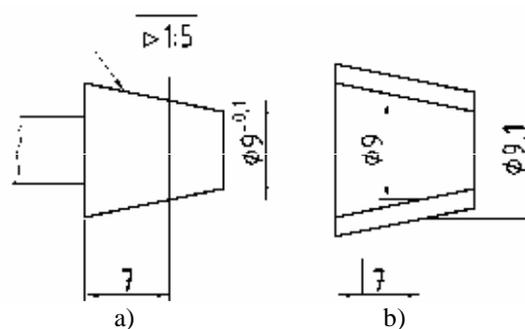
Figure 2. Method of normal conicalness
