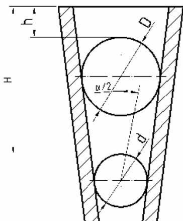
Figure 5. The method of the calibrated balls
