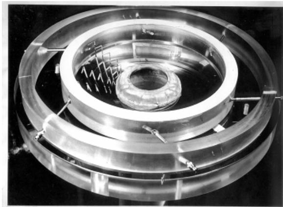
Figure 2. Experimental transparent model of the mill with supersonic jets
