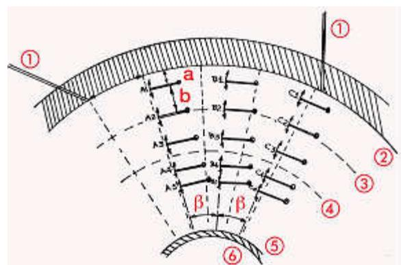
Figure 3. The positioning of the pressure sondes
