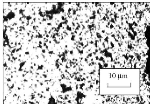
Figure 11. Microstructure of part produced by W-powder, noted F, with 2% paraffin
