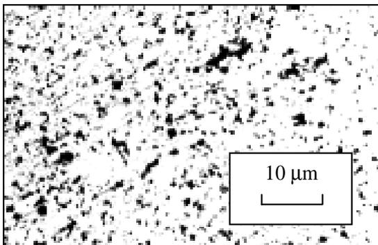
Figure 7. Microstructure of part produced by W-powder, noted B, with 1% paraffin
