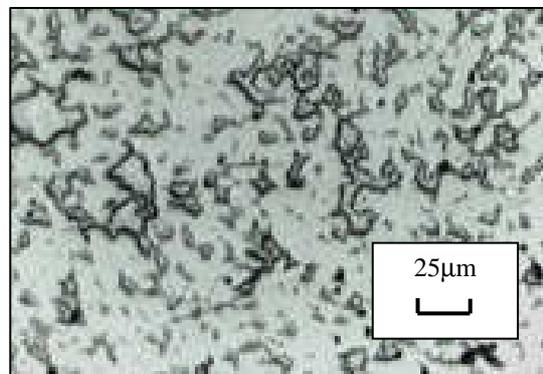
Figure 19. The microstructure of the pieces produced by W-powder, noted F, with 3% paraffin
