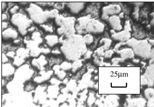
Figure 15. The microstructure of the pieces produced by W-powder, noted B, with 2% paraffin
