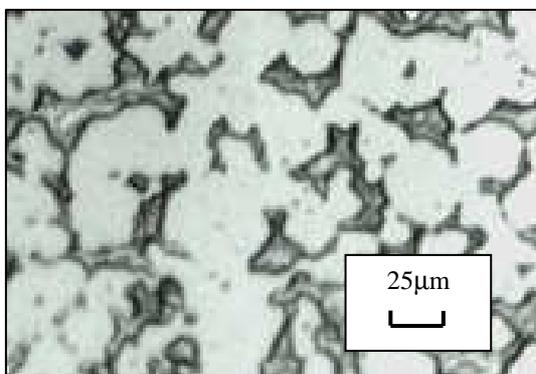
Figure 16. The microstructure of the pieces produced by W-powder, noted B, with 3% paraffin
