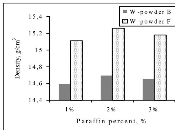
Figure 13. Final density obtained after copper infiltration
