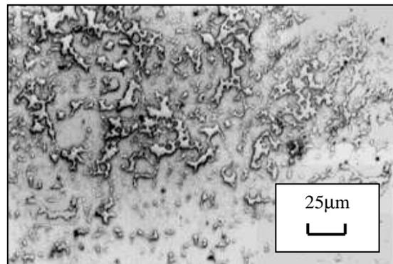
Figure 18. The microstructure of the pieces produced by W-powder, noted F, with 2% paraffin
