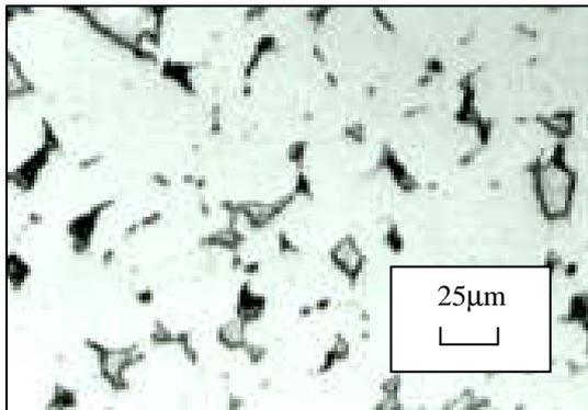
Figure 14. The microstructure of the pieces produced by W-powder, noted B, with 1% paraffin
