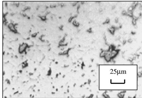
Figure 17. The microstructure of the pieces produced by W-powder, noted F, with 1% paraffin
