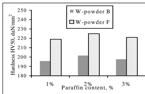
Figure 14. Final hardness obtained after copper infiltration
