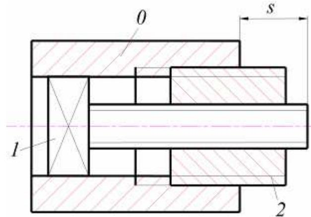
Figure 3. Closed differential screw mechanism with two threads
