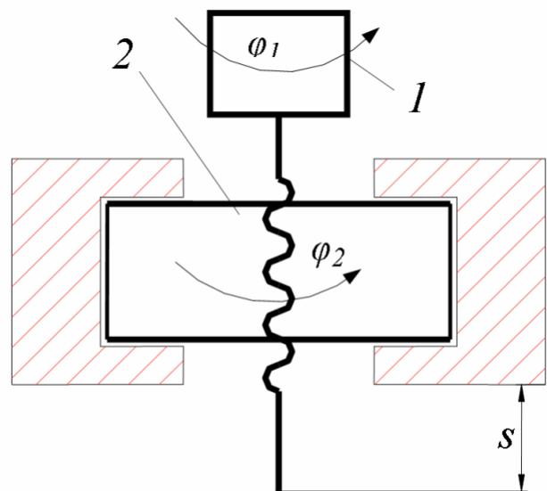
Figure 1. Differential screw mechanism
