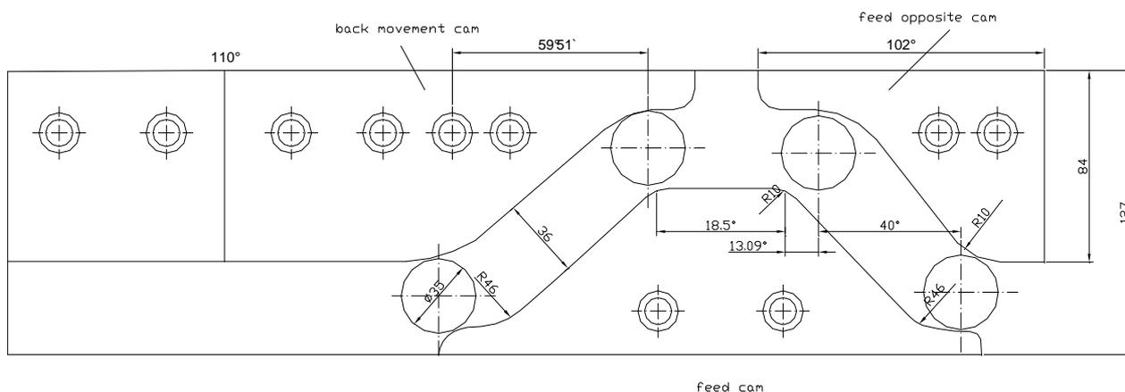
Figure 4. Cam set for longitudinal slide with independent feed, used for round profile thread Rd 8x2 left
