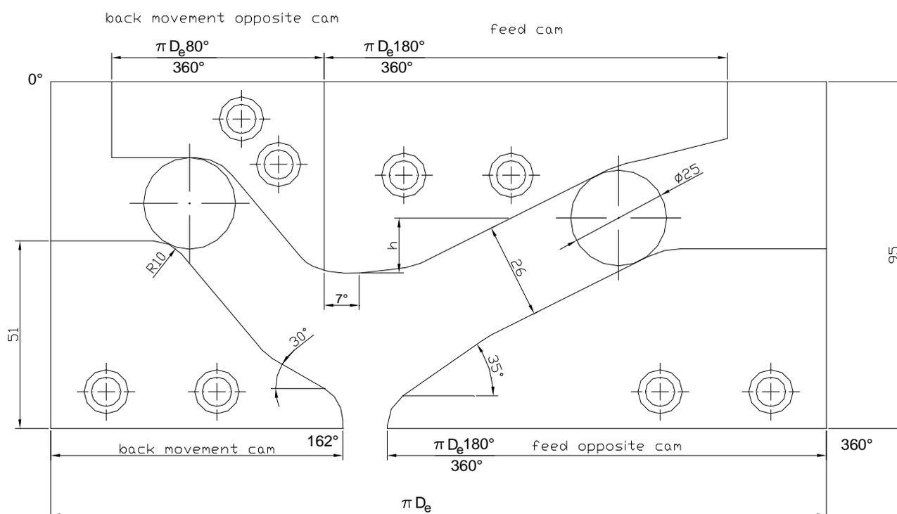
Figure 2. Cam set for radial slide
