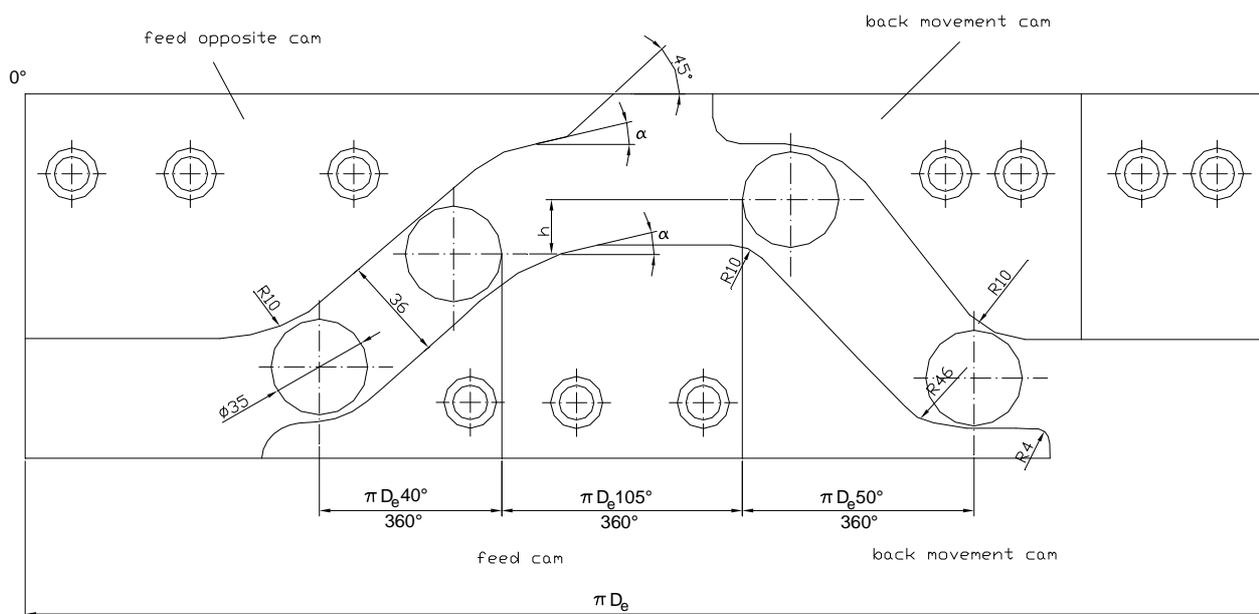
Figure 3. Cam set for longitudinal slide with independent feed
