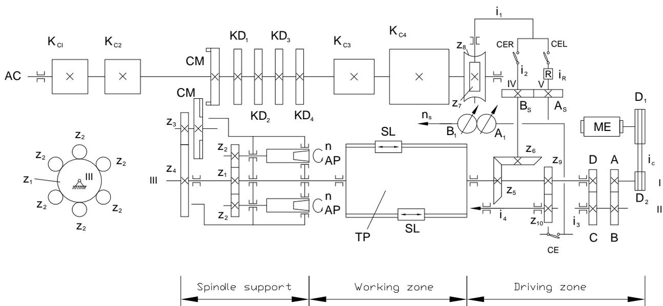
Figure 1. Kinematic scheme of multispindle automatic lathe
