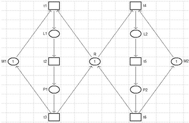
Figure 2. Petri net model for the manufacturing system
