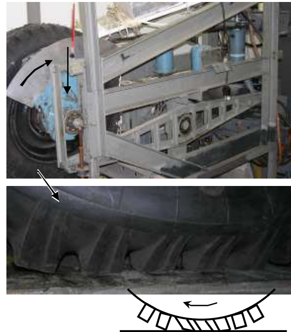
Figure 3. Static adhesion with contact area detail
