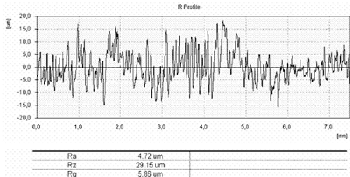
Figure 1. Surface roughness for shaft, at step 3
