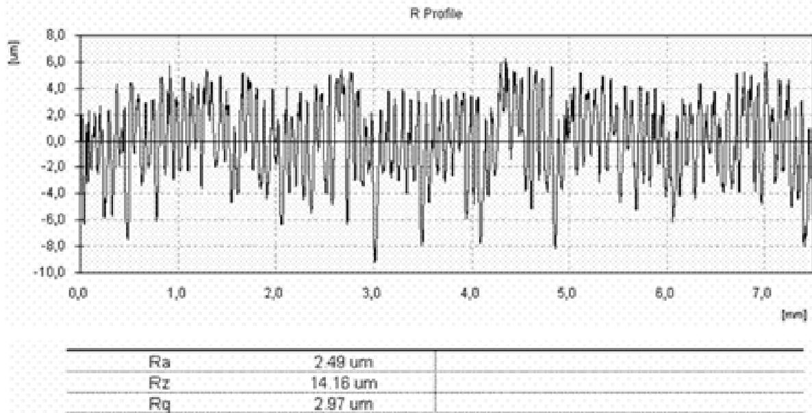
Figure 2. Surface roughness for bushing, at step 3
