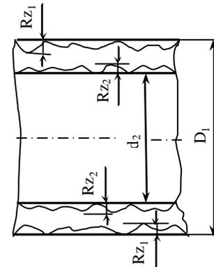
Figure 7. Scheme of surface roughness testing for shaft and bore
