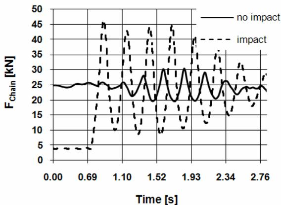
Figure 5. Forces in chain n1, model 1, lifting with and without impact, case B,  $v_c=0.16\text{m/s}$
