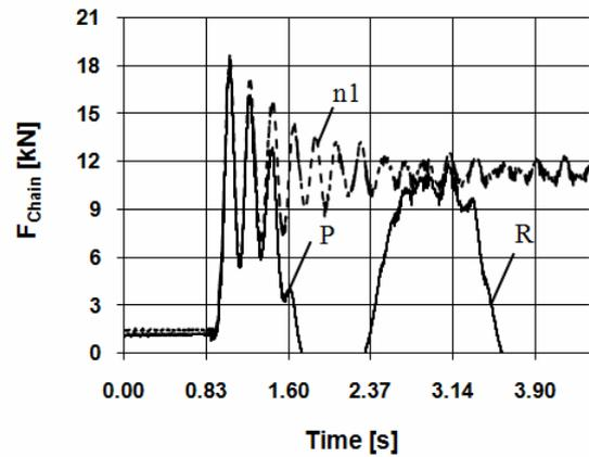
Figure 7. Forces in chain n1 and chain members P and R, model 2 lifting with impact,  $t_{\text{start}}=1.5\text{s}$ ,  $V_c=0.15\text{m/s}$
