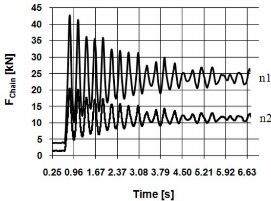
Figure 3. Forces in chains n1 and n2, model 1, case B,  $v_c=0.1\text{m/s}$
