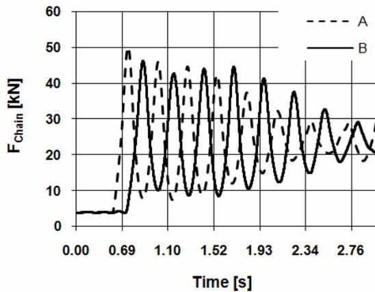
Figure 4. Forces in chain n1, model 1, cases A and B,  $v_c=0.16\text{m/s}$
