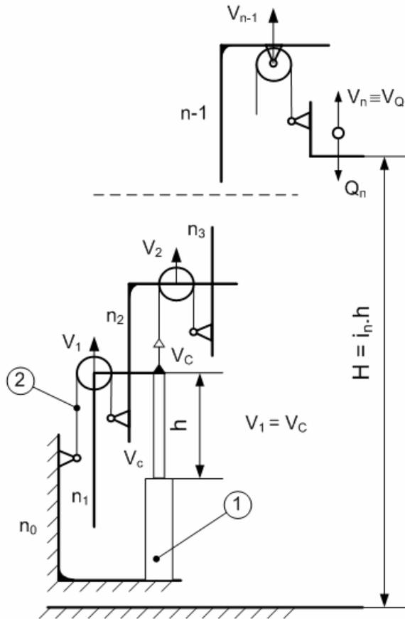
Figure 1. Lifting gear with one hydraulic drive
