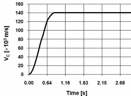
Figure 1. Hydraulic drive velocity,  $t_{start} = 0.84$ s,  $V_c = 0.14$ m/s
