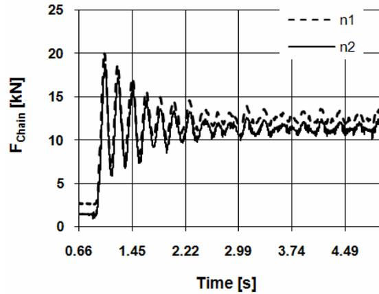
Figure 6. Forces in chains n1 and n2, model 2, lifting with impact,  $t_{\text{start}}=1.5\text{s}$ ,  $v_c=0.15\text{m/s}$
