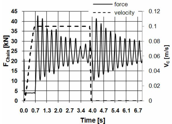
Figure 8. Force in chain n1, model 1, case A, sharp stopping  $t_{\text{stop}}=0.1\text{s}$
