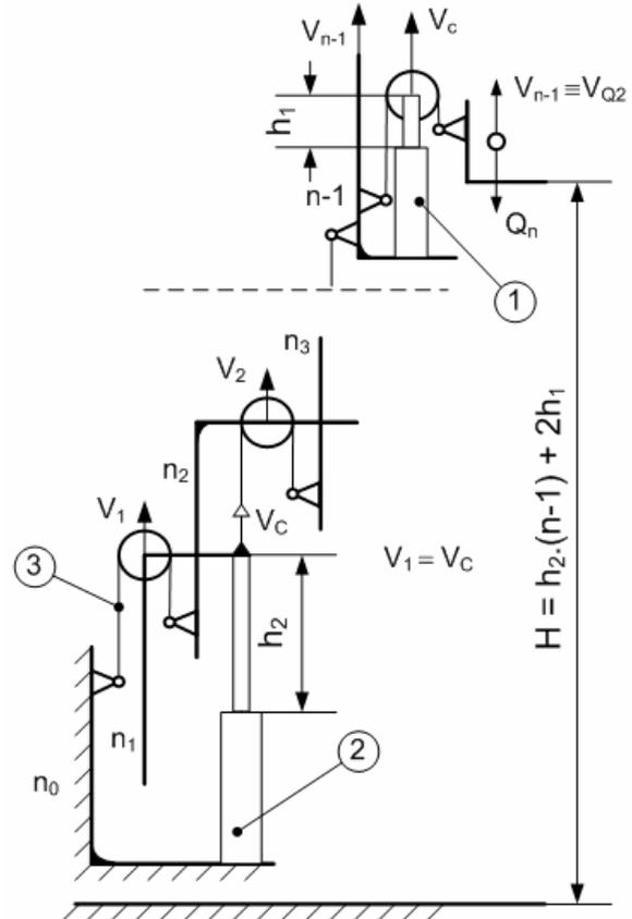
Figure 2. Lifting gear with two hydraulic drives
