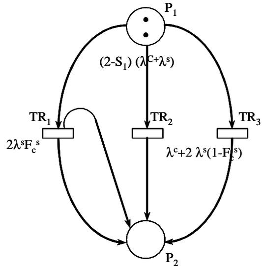
Figure 4. PN model for DACS structure of XPS-control system
