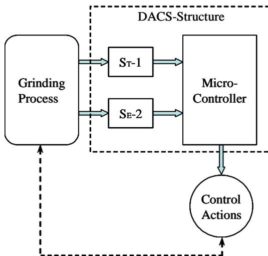
Figure 2. Structure of the DACS control system for XPS-grinding equipment
