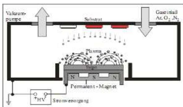
Figure 1. Principle of the magnetron sputtering process [10]
