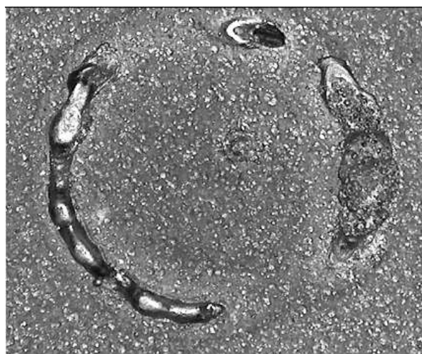
Figure 12. The laser radiation did not penetrate through the material
