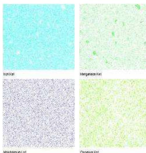
Figure 5. Iron and alloying elements distribution maps on the same surface of AM+B<sub>60</sub> steel
