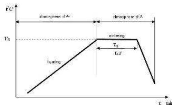
Figure 2. Sintering diagram
