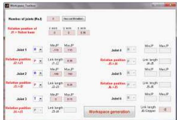
Figure 3. Data interface for SCARA structure
