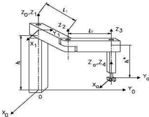
Figure 2. SCARA manipulator
