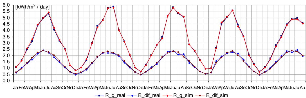
Figure 2. Estimated and real curves of the horizontal total and diffuse monthly average radiations for Braşov (R<sub>g</sub> – total radiation; R<sub>dif</sub> – diffuse radiation)
