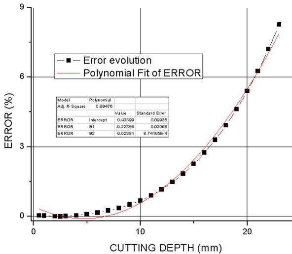
Figure 11. Channel error evolution (%) dependence on cutting depth (mm), for the cutting process with Rp3-type drill bit in OLC45 material
