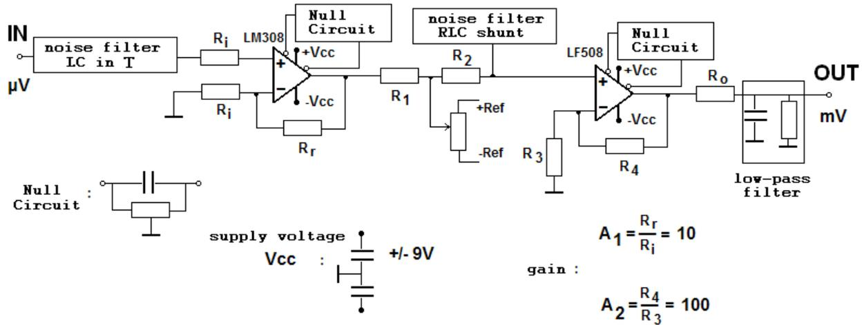
Figure 3. The DC amplifier schematic diagram
