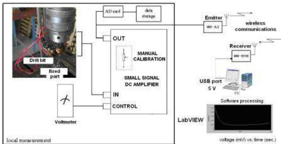
Figure 4. The system for monitoring the contact voltage with WN modules (schematic diagram)
