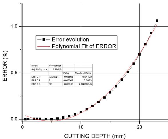
Figure 12. Channel error evolution (%) dependence on cutting depth (mm), for the cutting process with Rp5-type drill bit in OL50 material
