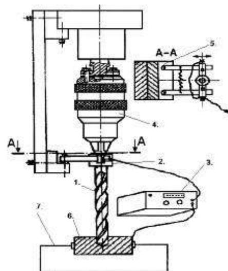
Figure 1. Assembly for monitoring the contact voltage during drilling
