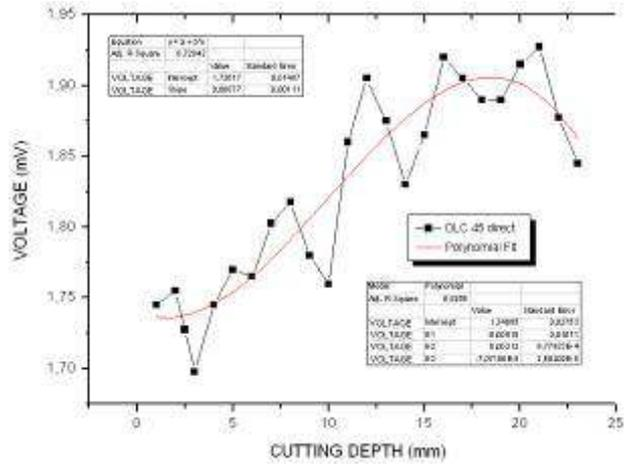
Figure 7. The average characteristic of the contact voltage for cutting OLC45 (local data storage)
