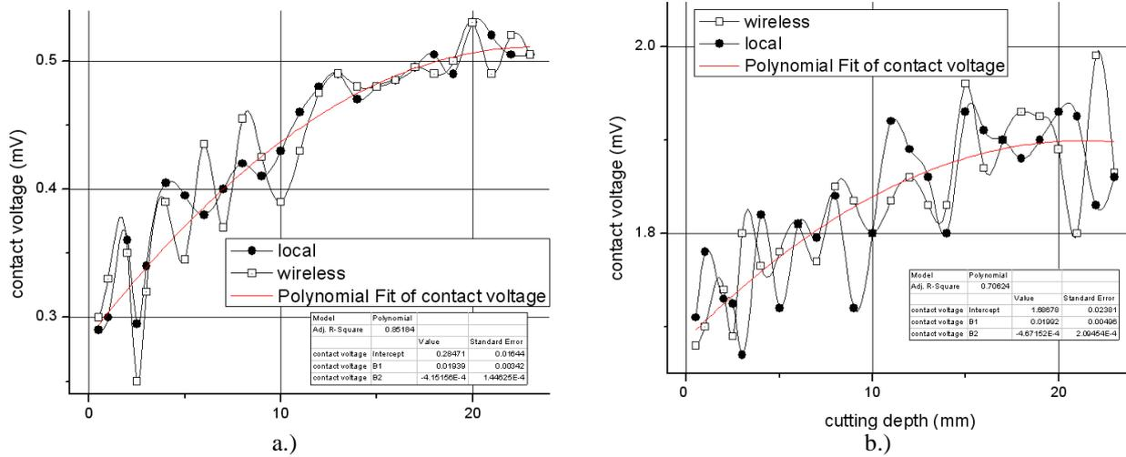
Figure 6. The influence of the cutting depth on the contact voltage during the cutting a.) OLC45 with drill bit from Rp3; b.) OL50 with drill bit from Rp5, using the two methods
