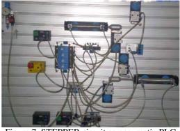
Figure 7. STEPPER circuit as pneumatic PLC
