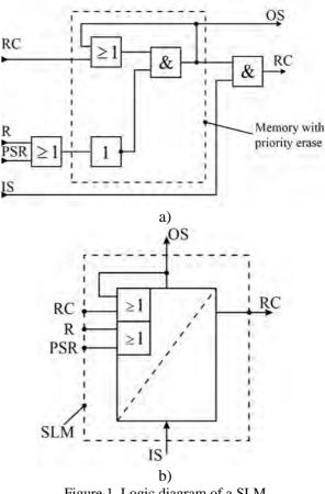
Figure 1. Logic diagram of a SLM
