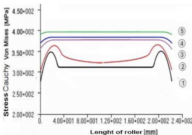
Figure 4. Graph of contact stress in roller depending on cavity-results obtained by finite element analysis
