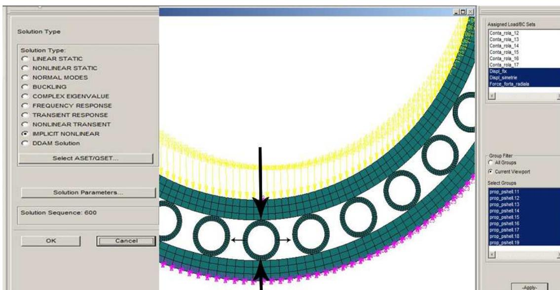
Figure 3. Loads distribution in roller – nonlinear method
