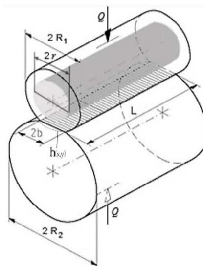
Figure 2. Contact roller-inner ring for hollow rollers
