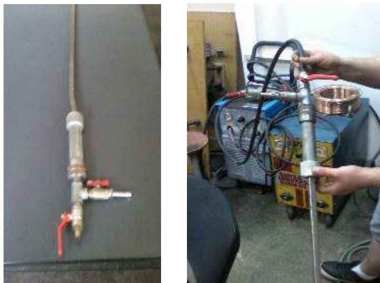
Figure 6. Port lance handle with lance and oxygen and metallic powder connection
