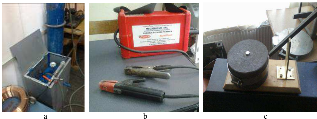
Figure 3. Overview thermal lance and metal powders cutting plant a - metallic lance with powders plant; b - power source for lance ignition; c - graphite and copper electrodes for lance ignition by Joule effect
