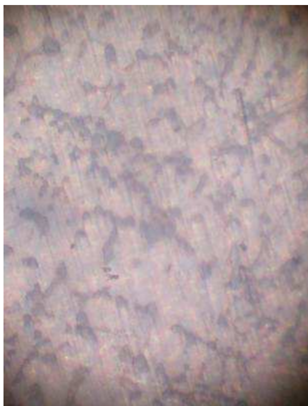
Figure 6. Alloy 1 after thermal isothermal treatment, with sustantation at 170 °C, with maintaining of 1 the hour. Attack HF, 200:1
