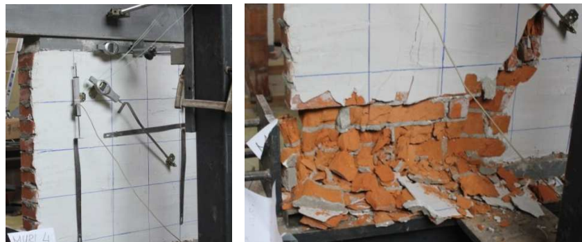
Fig. 7. Measurement points and failure mode of wall
