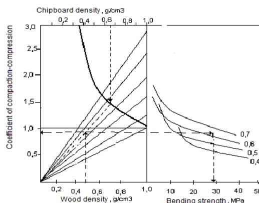
Fig. 2. Correlation of bending strength with wood and chipboard densities and coefficient of compaction-compression [5]
