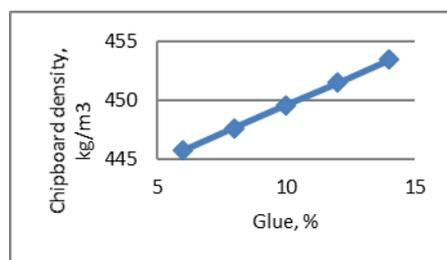
Fig. 5. The correlation between glue percentage and chipboard density
