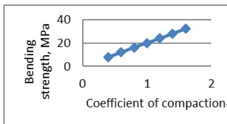
Fig. 1. Influence of the compacting- compression coefficient on the static bending strength
