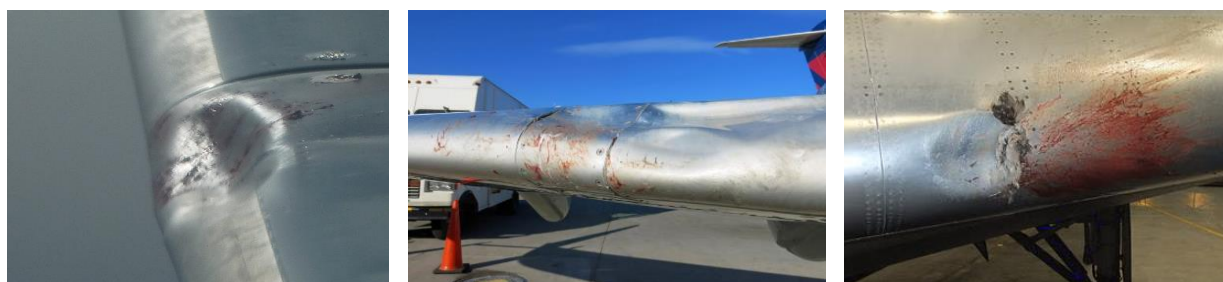
Fig. 3. Damage caused by birds [3, 4, 5]
