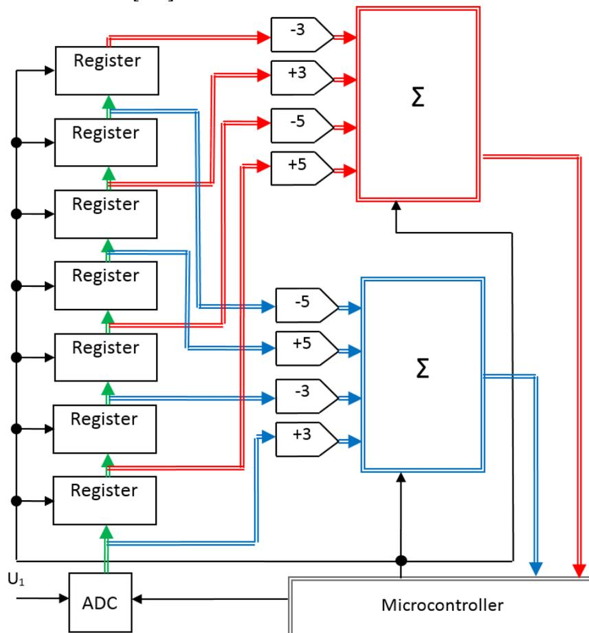
Fig. 5. Possible scheme for realization of the phase meter on separate discrete elements
