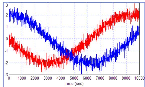
Fig. 2. The result of calculating of the difference frequency with the relations (1), (2) from the signal shown in Figure 1
