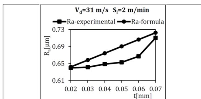
Fig. 8. The dependence of the roughness  $R_a$  at grinding with  $V_d = 31$  m/s, and  $S_l = 2$  m/min
