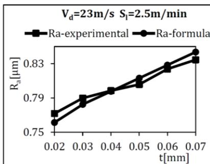
Fig. 4. The dependence of the roughness  $R_a$  at grinding with  $V_d = 23$  m/s, and  $S_l = 2.5$  m/min
