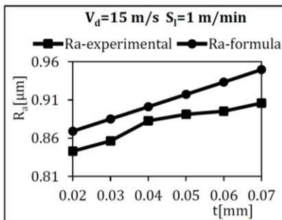
Fig. 2. The dependence of the roughness  $R_a$  at grinding with  $V_d = 15$  m/s, and  $S_l = 1$  m/min
