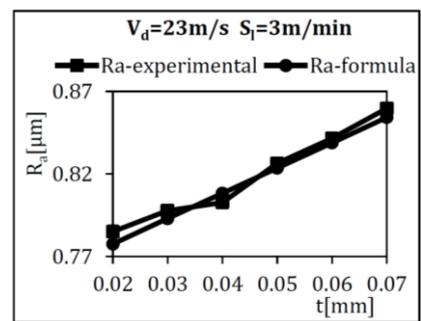
Fig. 5. The dependence of the roughness  $R_a$  at grinding with  $V_d = 23$  m/s, and  $S_l = 3$  m/min
