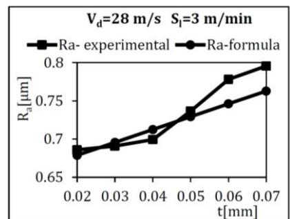
Fig. 7. The dependence of the roughness  $R_a$  at grinding with  $V_d = 28$  m/s, and  $S_l = 3$  m/min
