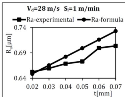
Fig. 6. The dependence of the roughness  $R_a$  at grinding with  $V_d = 28$  m/s, and  $S_l = 1$  m/min
