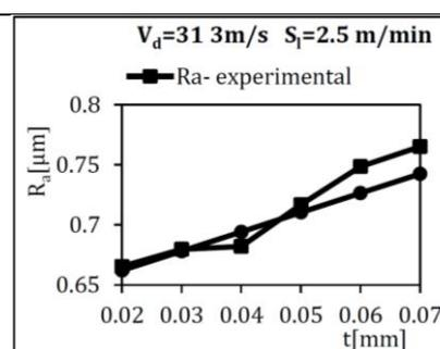
Fig. 9. The dependence of the roughness  $R_a$  at grinding with  $V_d = 31$  m/s, and  $S_l = 2.5$  m/min
