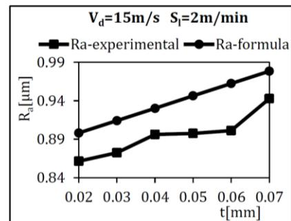
Fig. 3. The dependence of the roughness  $R_a$  at grinding with  $V_d = 15$  m/s, and  $S_l = 2$  m/min
