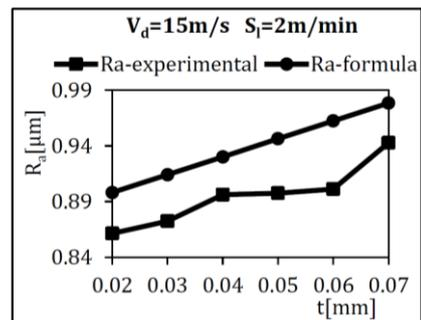
Fig. 3. The dependence of the roughness  $R_a$  at grinding with  $V_d = 15$  m/s, and  $S_l = 2$  m/min
