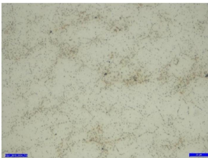
Fig. 3. 40Cr130 hardened to 1050 °C, held for 1.5 hours and tempered at 510 °C. Attack Nital. 1000:1
