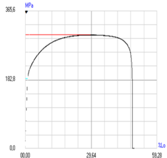
Fig. 4. Variation graphic of the tensile strength for CC 45 steel in the presence of vibrations
