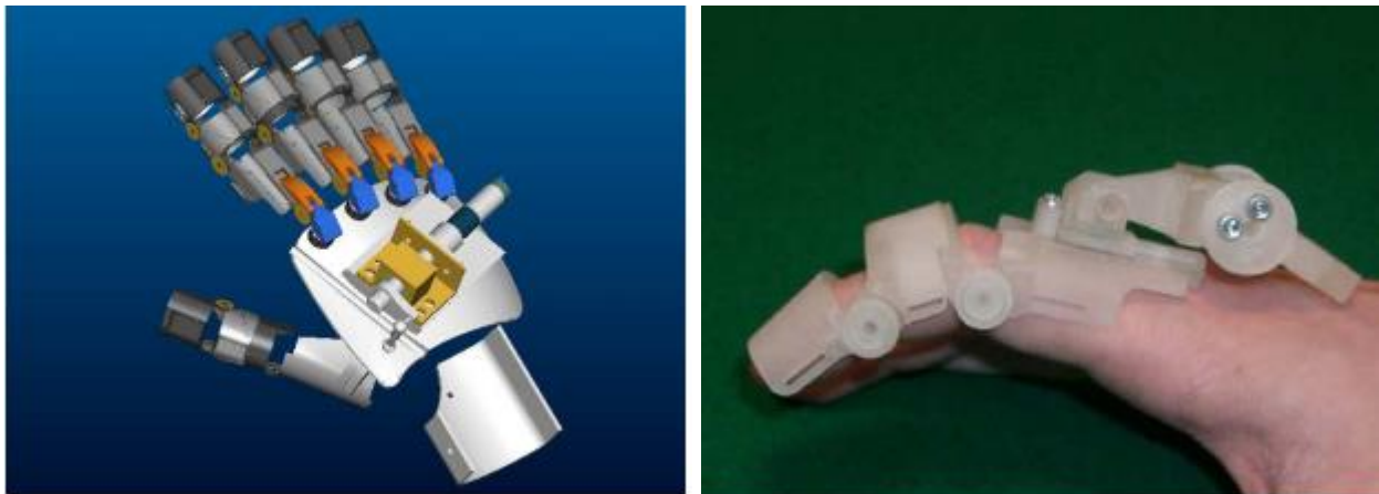
Fig. 2. Schematic (left) and prototype (right) of the HandExos rehabilitation device
