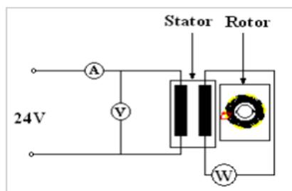
Fig. 6. Simplified diagram of the installation used to examine cast rotor squirrel cages
