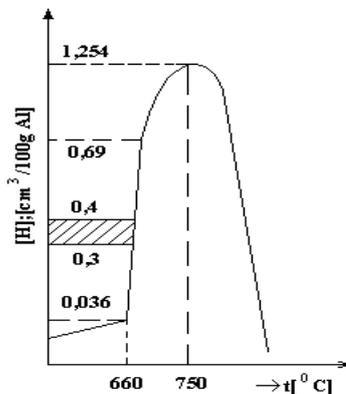
Fig. 3. Representation for assessing the tendency of bubble formation in castings according to the hydrogen content of the liquid metal [8, 9]
