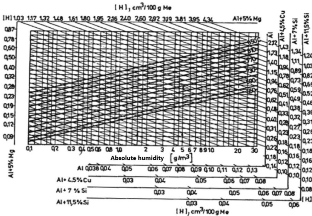
Fig. 2. Nomogram for the assessment of the maximum probable hydrogen content of liquid aluminium alloys, according to the elaboration conditions [8, 9]
