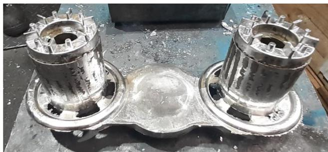
Fig. 4. Rotor squirrel cages after casting with the casting grid
