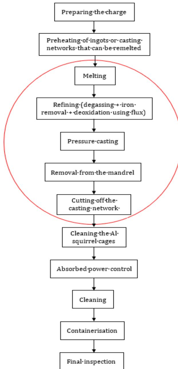
Fig. 1. The process flow for casting aluminium rotors at Electroprecizia Electrical Motors Săcele
