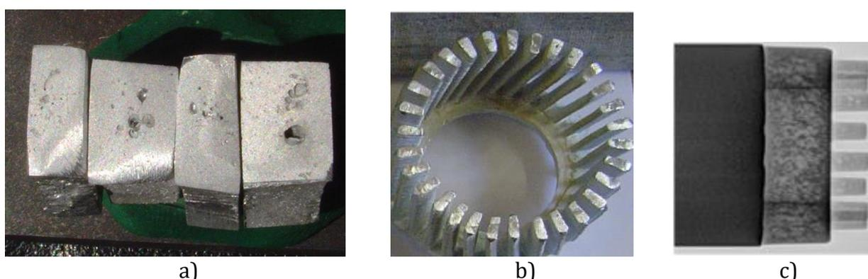
Fig. 5. Voids in the rings of the rotor squirrel cages (a, c) and in the bars inside the laminations (b)
