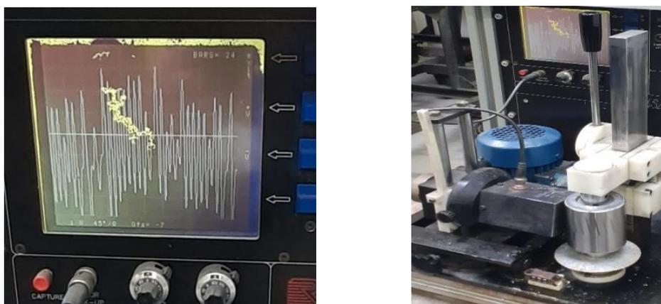
Fig. 7. The diagram recorded upon examining the integrity of the bars inside the rotor (laminations) on the RISATTI device
