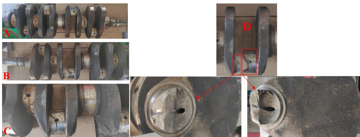
Fig. 1. A) – Crankshaft; B) – Broken crankshaft; C) – Breakage detail D) The appearance of the fracture surface
