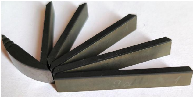
Fig. 2. PCD sliced in pieces by using wire EDM
