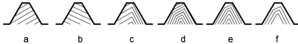
Fig. 3. Machining schemes with different attack cone geometries, specific to taps without flutes
