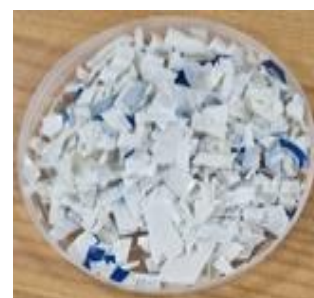
Fig. 3. Short fibres of LDPE
