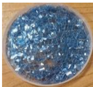
Fig. 2. Short fibres of PET
