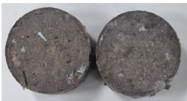
Fig. 5. Bentonite and clay composite reinforced with PET fibres
