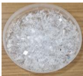
Fig. 1. Short fibres of PP
