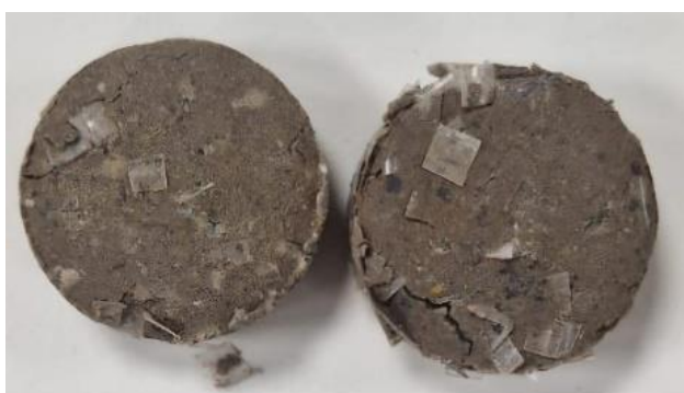
Fig. 4. Bentonite and clay composite reinforced with PP fibres
