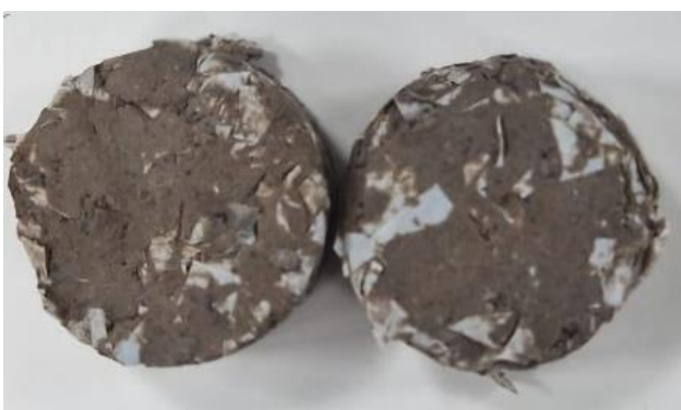
Fig. 6. Bentonite and clay composite reinforced with LDPE fibres
